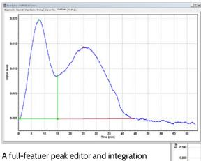
A full-featuer peak editor and integration package is included with the AutoChem II. This easy-to-use package provides a rapid method for evaluating common temperatureprogrammed and dynamic adsorption data.
