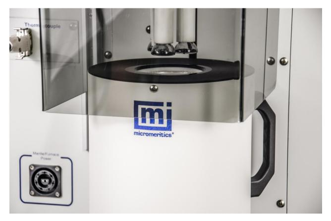
To avoid obstruction with the dewar safety shield, the dewar must be installed with the Micromeritics logo facing forward. This position will place the dewar handle close to the analyzer front panel.
