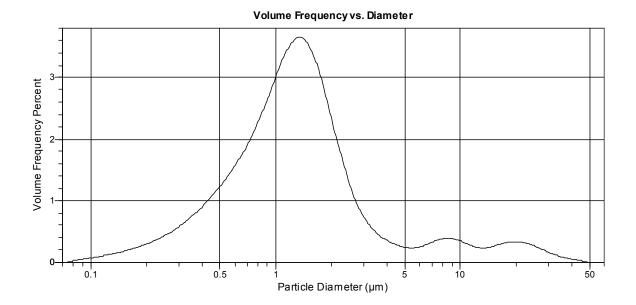
Figure 3. Alumina sample analyzed at 10.9% obscuration and 5% minimum signal fraction.
